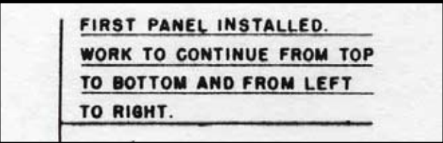
Drawing EM-02-L-32.1 from the Lustron Erection Manual, showing the completed left elevation. A note in the upper left (enlarged here below the drawing) indicates the starting point for hanging the exterior panels on this elevation. —Courtesy of the Arlington County, Virginia, Historic Preservation Program
